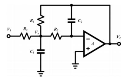
Figure 1 - Rauch Filter Circuit
